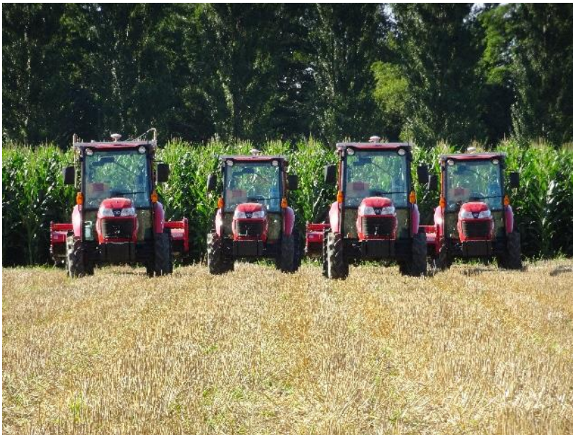
Cooperative operation of an unmanned tractor (HP University of Hokkaido)
